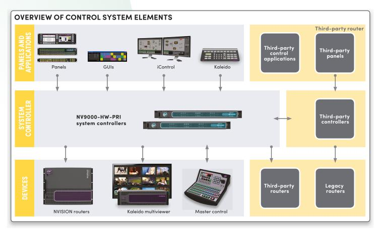
The NV9000 is a complete and agnostic router control system that fully supports any of the NVISION control panels and all legacy NVISION routers, as well as interfacing with the most popular routers and control systems in the market.
