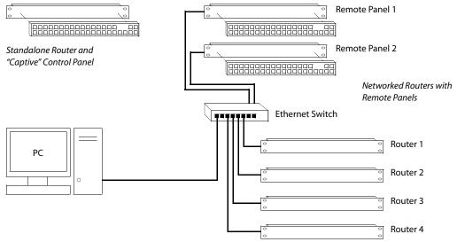
Figure 12-3. Standalone Router vs. a Network of Routers
