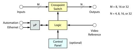
Figure 12-20. Block Diagram of the Analog Video Router
