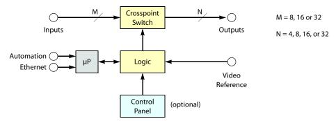
Figure 12-21. Block Diagram of the AES Router
