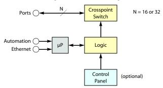
Figure 12-23. Block Diagram of the Machine Control Router
