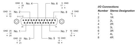
For  $16 \times 16$  routers, the connectors provide inputs (or outputs) 1–8, 9–16, 17–24, and 25–32, respectively, and are labelled that way on the rear of the router. Inputs (and outputs) are treated as 16 stereo pairs.
