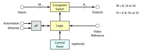
Figure 12-22. Block Diagram of the Analog Audio Router
