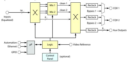
Figure 12-18 shows a simplified view of the CQX digital video router:
