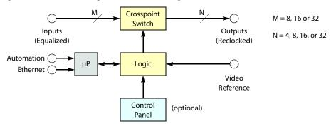
Figure 12-17. Block Diagram of the Digital Video Router
