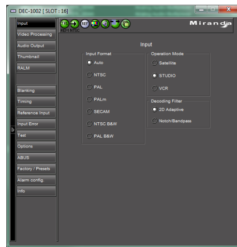
Example of a control panel for a DEC-1002 Analog Video to SDI Encoder
