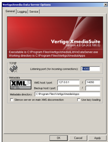
Figure 3-14. The Data Server Control Panel
