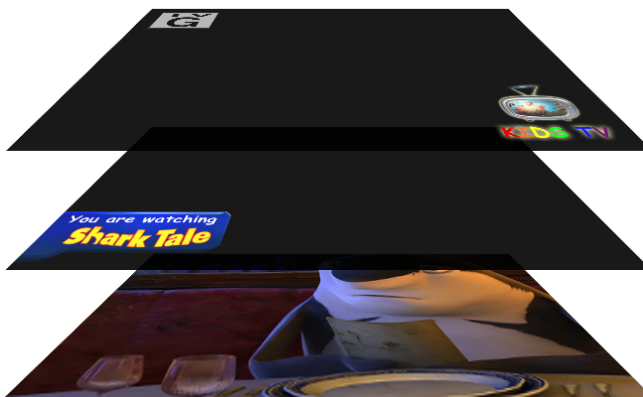
Figure 2-6. The Vertigo XG supports the production of multi-layered graphics
