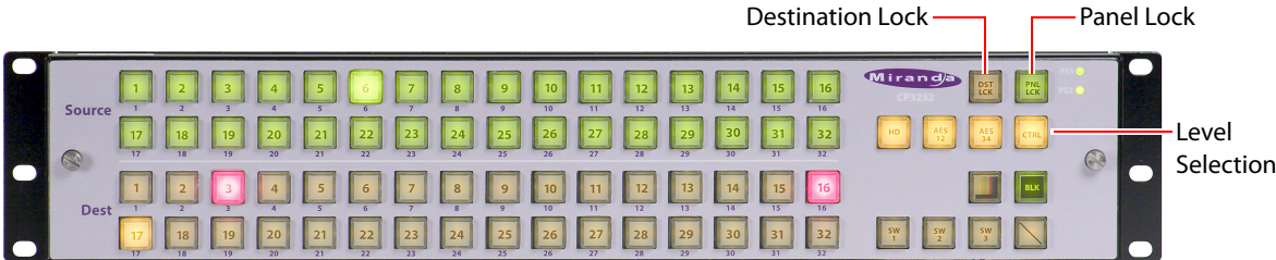
Fig. 2-29: Front view of the CP3232 Control Panel
