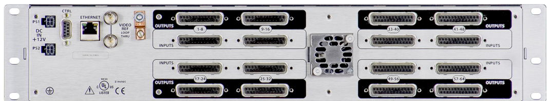
Fig. 2-13: Rear View of the CR1616-AA Analog Audio Router
