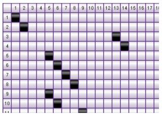
Asynchronous AES takes occur in adjacent pairs. This diagram illustrates, for example, that inputs (13,14) are taken to outputs (3,4).
