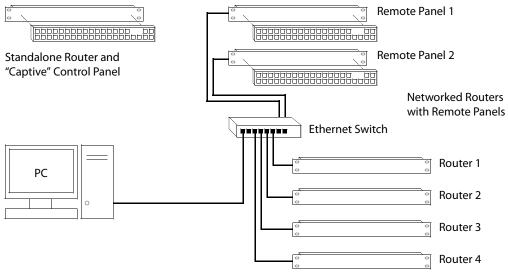
Fig. A-3: Standalone Router vs. a Network of Routers
