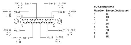
For 16×16 routers, the connectors provide inputs (or outputs) 1–8, 9–16, 17–24, and 25–32, respectively, and are labelled that way on the rear of the router. Inputs (and outputs) are treated as 16 stereo pairs.
