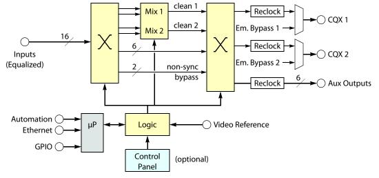
Figure A-20 shows a simplified view of the CQX digital video router:
