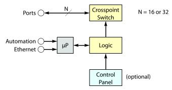
Fig. A-26: Block Diagram of the Machine Control Router
