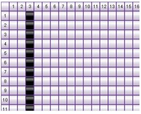
For asynchronous AES routers, stereo input pair *n* is connected to all stereo output pairs. The pattern is vertical, but occupies two columns in alternation. For synchronous AES routers, the result is a single column for any input you choose:
