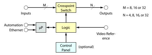
Fig. A-23: Block Diagram of the Analog Video Router
