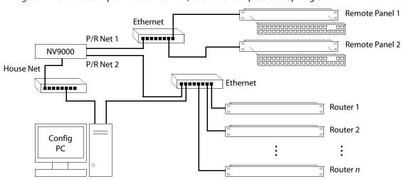
Figure A-4 shows a sample NV9000 network, one of several possible topologies:
