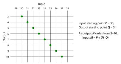
A reverse diagonal take connects inputs *M* to outputs *N*, in *descending* order, given an input starting point that you specify:
