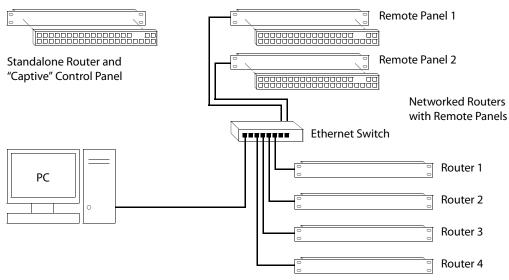
Fig. 1-1: Standalone Router vs. a Network of Routers
