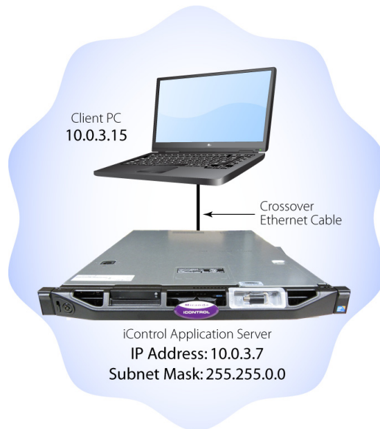
Connection between client PC and Application Server
