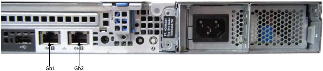
Rear view of R310 Application Server, showing logical ports eth0 and eth1 (physical ports Gb1 and Gb2, respectively)
