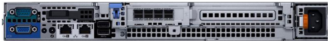
Rear view of R310 Application Server, showing logical ports eth0 and eth1 (physical ports Gb1 and Gb2, respectively)
