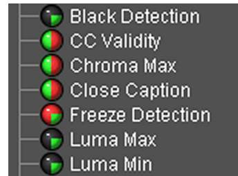
Alarms in the GSM showing combined components (current, latched, and acknowledged)
