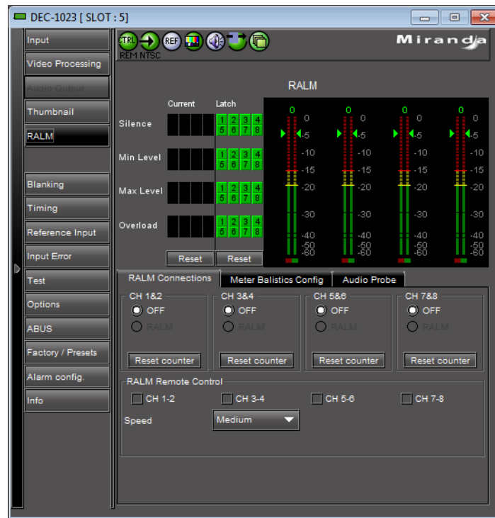
Example of a control panel showing RALM settings
