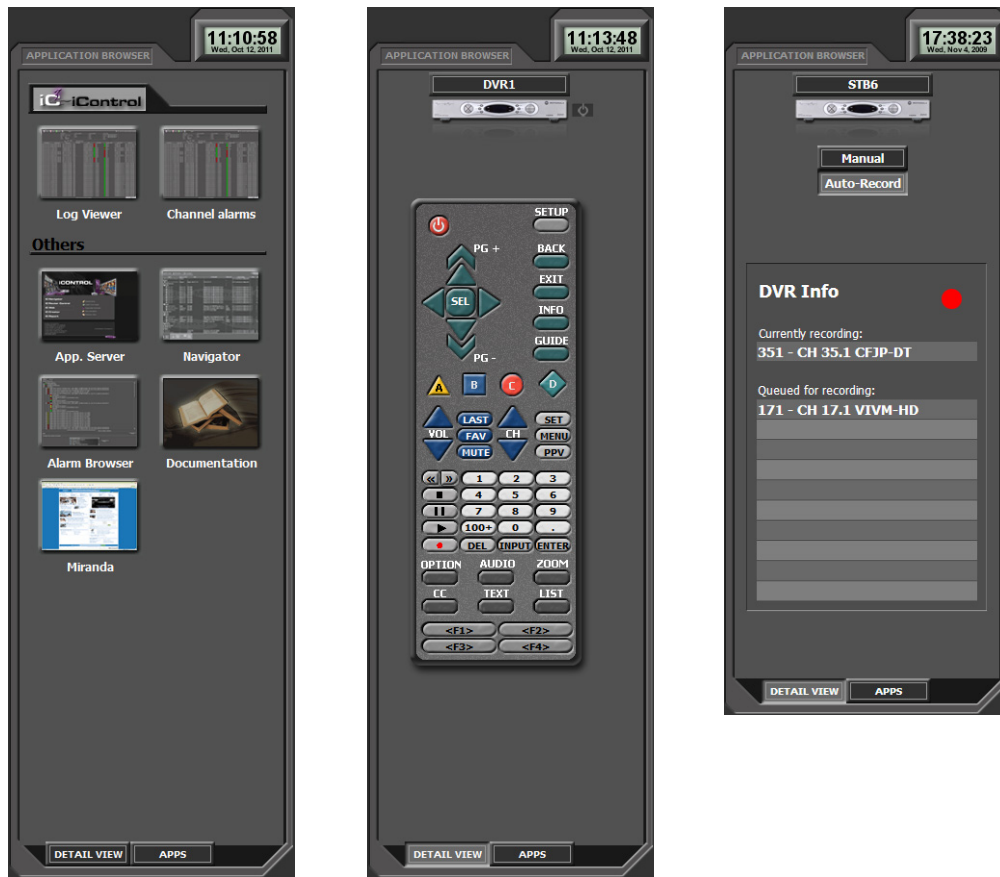
iControl Edge user interface (Application Browser area: Application Selector, Soft Remote, and DVR Info)
