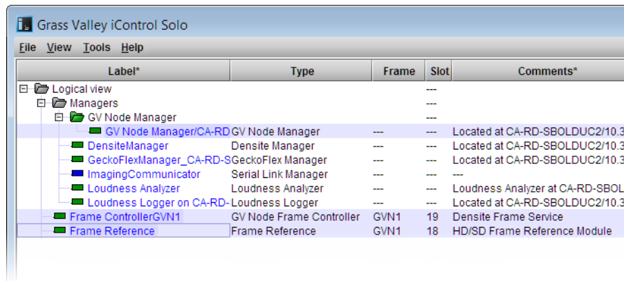
Logical view showing GV Node Manager, Frame Controller, and Frame Reference
