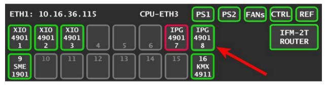
To access the menu for this IPG-4901, touch the virtual button corresponding to the card (identified by card type and slot number) in the home screen.
