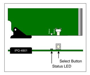
Figure 1-3 Front card-edge layout
