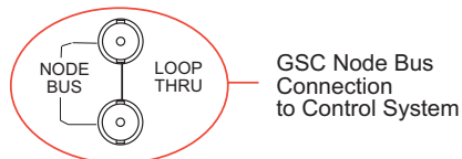
Figure 3-15. GSC Node Bus Connection to Control System (Rear View)
