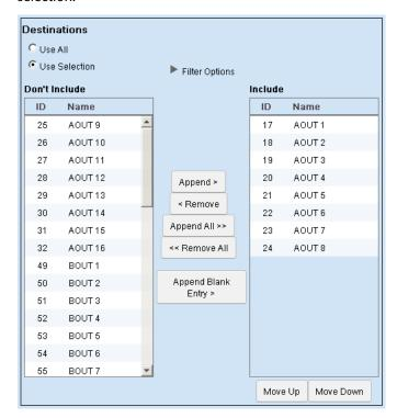
The 'Use Selection' fields include filtering options. See <u>Filter Options for Destinations</u>, following. The items on the left — under "Don't Include" — are the destinations that are *not* used in the matrix view.
