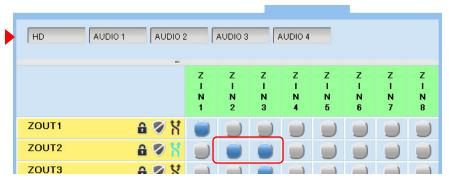
When you display only level AUDIO1, the display shows that it is from ZIN3 (for ZOUT2):
