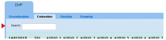
You can place text in this field to limit the number of rows that are displayed. Only those rows in which the search text appears — in any column — are displayed.
