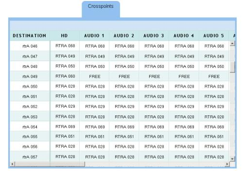
Thus, each field to the right of the destination column is a source on the level indicated by the column header. If there is no source on a particular level, the field displays a dash.
