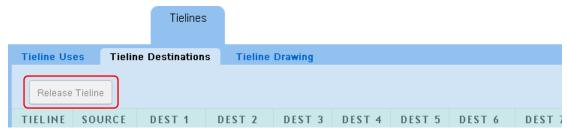
When the 'Release Tielines' button is enabled, you can release tielines. To do so, select a tieline path in the uses table and click the button. the software displays a warning:
