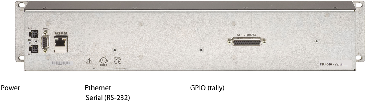
Power — Ethernet — Serial (RS-232) — GPIO (tally) Fig. 2-2: NV9640 Rear
