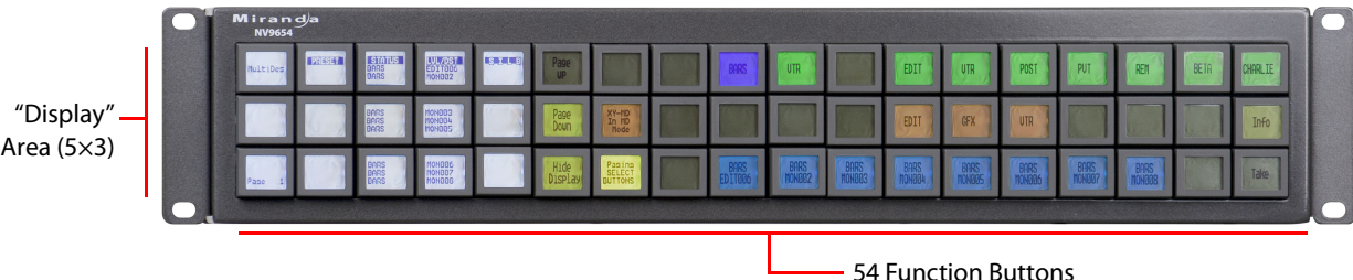
Fig. 2-1: NV9654 Front View
