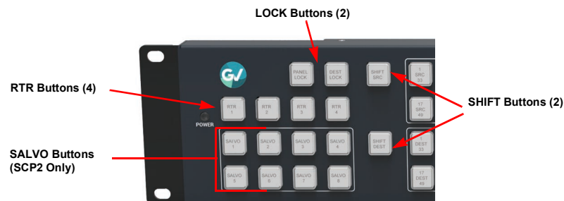
Fig. 4-2: Sirius Control Panel Function Buttons
