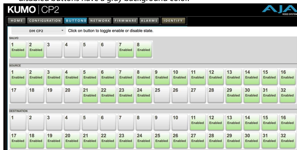
Fig. 4-6: Sirius SCP2 Configuration with Disabled Buttons
