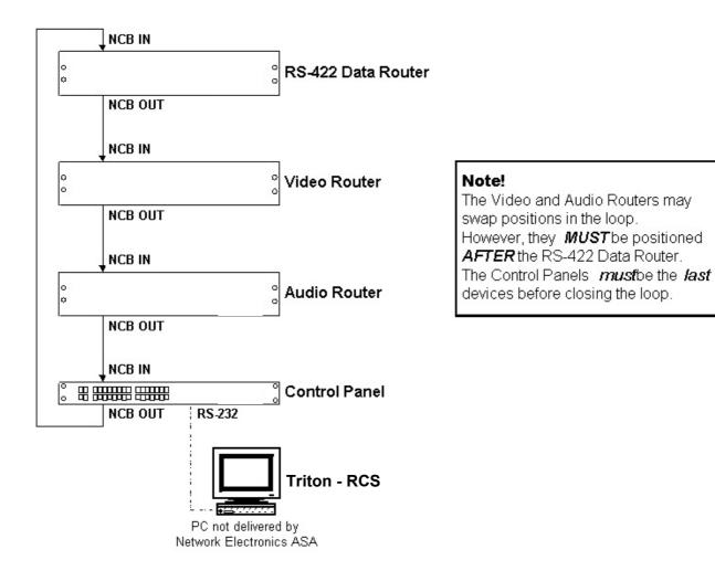
• Complete the Control loop, by connecting all Control bus connections to all Triton devices, before powering up any Triton device.
