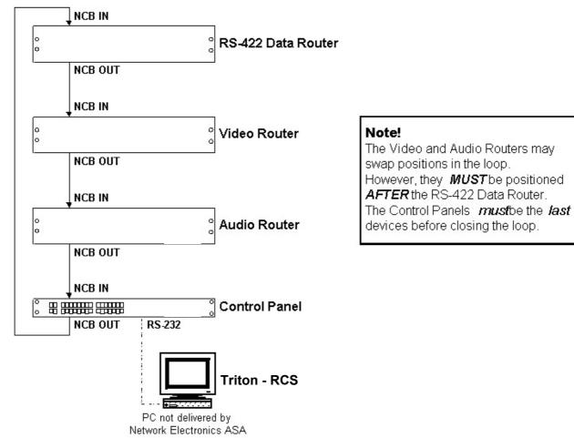
Complete the Control loop, by connecting all Control bus connections to all Triton devices, before
