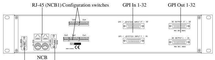
Power connector RS-232 port, connection via 0-modem cable to Second GPI Panel
