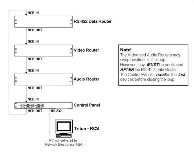
*Complete the Control loop, by connecting all Control bus connections to all Triton devices, before powering up any Triton device.*
