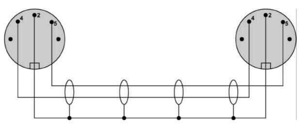
Pin 1 = Not Connected Pin 2 = shield Pin 3 = Not Connected Pin 4 = data Pin 5 = data
