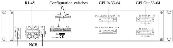
Power connector RS-232 port, connection via 0-modem cable to Input Selection Panel
