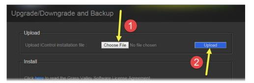
System Response: The upgrade package is uploaded to the Application Server. A progress bar displays the upload progress.
