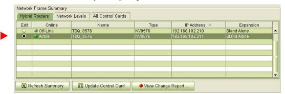
If you are updating an expanded NV8576-Plus, you must select **Card A** of the master frame. MRC will present a dialog asking you to identify the slave frame. Choose the slave frame in this dialog. (But do *not* select the slave frame in the 'Control Cards' tab at the bottom of the 'Module Types' page!)
