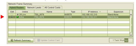
If you are updating an expanded NV8576-Plus, you must select **Card A** of the master frame. MRC will present a dialog asking you to identify the slave frame. Choose the slave frame in this dialog.
