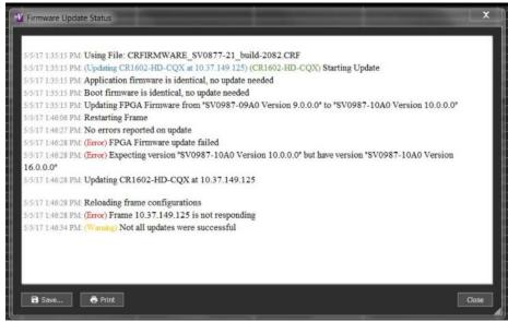
To make sure the update was successful; select the "Firmware Updates" option under the "Administrative Tools" left side bar of the CRSC application. Select the CQX router and note the part number should display SV0987-10A v16.0.0.0 as shown in the image below.
